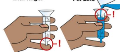
3. Remove finger from nozzle as you start the stopwatch
